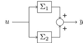
Fig. 1. Parallel interconnection of two EIP systems.
