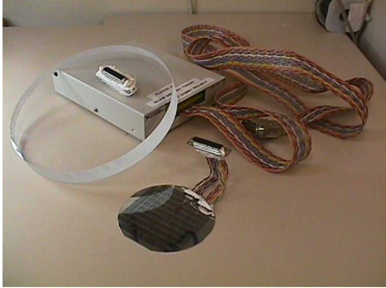
Figure 5.12: Picture of data acquisition system, including clear \text{XeF}_2 lid with electrical vacuum feedthrough.
